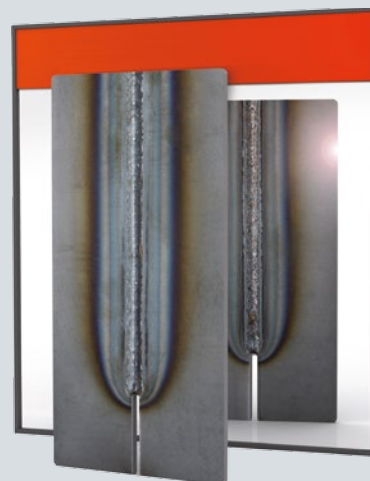
What is mainly crucial for root welding is what is otherwise not seen: Shown as a mirror image: weld front side (left) and weld rear side (right).
