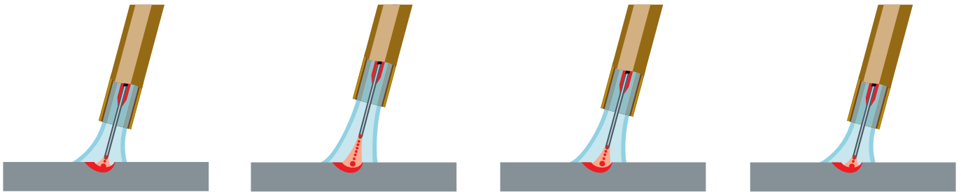
The welder can react much more easily to arising conditions by adjusting the distance of the torch.
