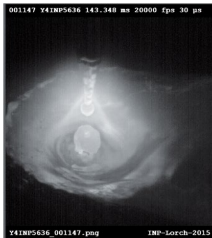
Fig. 2: The primary droplet has detached, allowing the secondary droplets to form.
